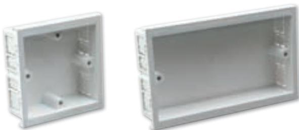
Outlet boxes for switches and sockets accredited to BS 4662; white, for clip-on mounting, lugs with brass inserts M 3.5mm, with knock-out cable entries.
