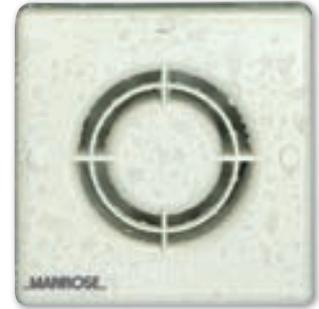
Suitable for mounting within the splash area of a shower or bath (where current regulations prevent the use of conventional fans), the 12 Volt fan is a standard model manufactured with a 12V - 50Hz shaded pole motor. The transformer and switching mechanism is mounted remotely either in the roof space or high on the ceiling next to the pullcord switch.
