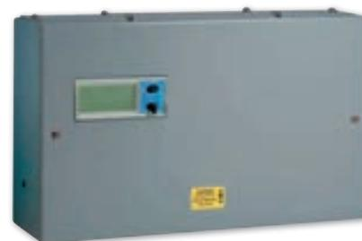
Eaton's Memshield 3 meter packs provide simple integration with matched aesthetics. Split metering for separate small power and lighting has been added to the range to meet the needs of the L2 Regulations introduced in England and Wales in 2006. The meters provide a pulsed output for kWh and display other useful parameters, including line voltage and current. Modbus versions are also available and provide remote access to additional electrical parameters.
