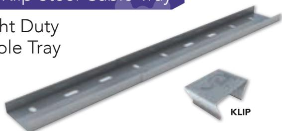
All light duty tray lengths up to and including KLLD225T come complete with swaged end for ease of coupling and to eliminate the need for couplers. KLLD300T and above require the use of couplers. A range of gauges are available on request. Pre-galvanised to BS EN 10346:2009.
