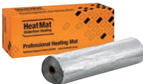
The 150W Combymat system is quick and easy to install, without the need for levelling compound. This system can provide sole source heating under a wide range of floor finishes including floating laminate or engineered boards and when combined with overlay boards carpet or vinyl. All Combymats need to be fitted onto 6mm foam underlay using aluminium tape to ensure heat spreads evenly across the floor.
