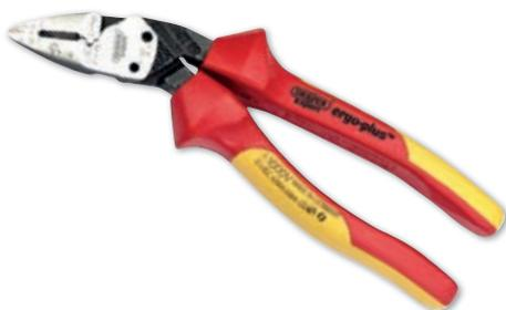
Expert quality, special steel hardened and tempered with cutting edges separately induction hardened. Ergonomic shape of head and handles allow user to access difficult working areas and still keep a tight grip on the workpiece.
