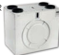
Xcell MVHR mechanical ventilation with heat recovery (MVHR) units with summer bypass. Features low energy EC motors, long life G4 filters and a counterflow heat recovery cell up to 90% efficient. Has a lightweight EPP construction that allows for floor or wall mounting.
