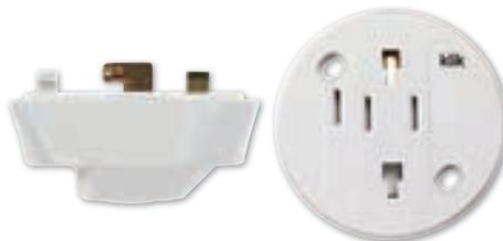
Klik 6A pre-wired plug in ceiling roses are used to connect luminaires to a fixed wiring installation. Auxiliary contact available, a typical use is for emergency lighting.
