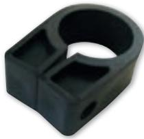
A comprehensive range of single fixing cable cleats to provide a simple, but strong means of securing cables. Suitable for use with cables or pipes up to 50.8mm in overall diameter.
