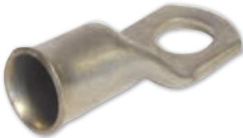
Manufactured from seamless copper tube to BS2871/C4106, bell mouth entry, inspection hole, internal barrel diameter suit cables as defined in BS6360, Comply to BS EN 61238-1-2003 & IEC 61238-2003.
