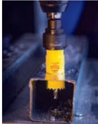
The Fast Cut saw combines a new tooth material, with enhanced heat and wear resistance, and a new tooth design, providing a smoother, faster cut on a wide range of materials, when compared against the previous Constant Pitch saw.
