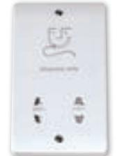
Click® dual voltage shaver outlets incorporate a double wound isolating transformer rated 20Va at 230V or 115V and meets BS EN 61558-2-5: 1998 making it safe for use in bathrooms. Shaver outlet is not continuously rated and therefore not suitable for use as a permanent charging outlet.
