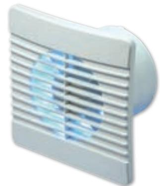
100mm and 150mm panel axial fans for bathrooms, cloakrooms and kitchens. Slim profile only 15mm. Suitable for wall or panel mounting using the appropriate fixing kit. Provides required performance of 54m<sup>3</sup>/h (15l/s) - bathrooms and 216m<sup>3</sup>/h (60l/s) - kitchens to comply with the Building Regulations (Document F).
