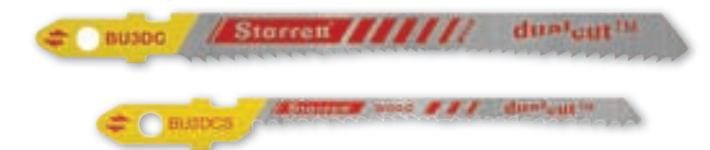
The two new wood-cutting saw designs with teeth in both directions offer a burr-free cut on both sides. Bi-metal unique saw technology provides 170% greater resistance to tooth breakage, longer life and a lower cost per cut than other blade manufacture techniques.
