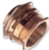
Brass indoor and outdoor glands suitable for all types of flexible wire braided cable such as CY and SY. The gland provides an environmental seal on the cable's outer sheath and internal mechanical retention of wire braid for electrical continuity. Gland complete with steel locknuts and brass washers.
