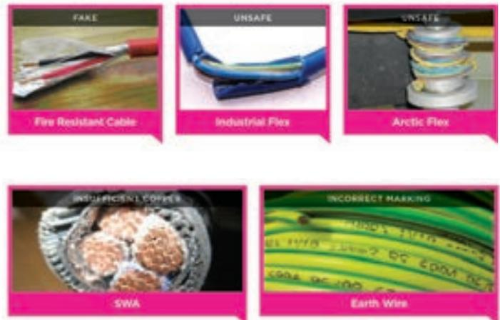
deteriorates the insulation and sheathing materials: they crack and fall off exposing the live conductors at a high temperature. This is a recipe for a fire, a fire that could start out of sight in a void in living accommodation for instance. Purchase cable you trust from a supplier you trust.
