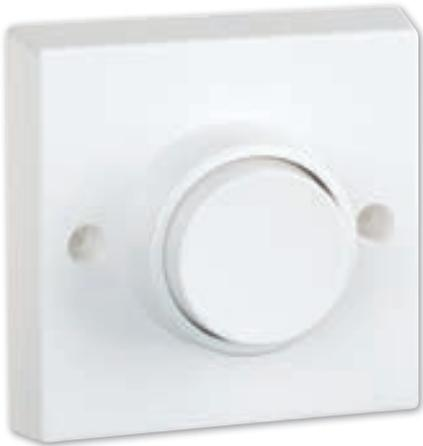
Columbus® Electronic Timer is an easy to fit and cost effective way of automatically turning lighting off after a set period of time. Pushing the button switches the switch and activates the time delay, which can be set at installation anywhere between 20 seconds and 25 minutes.
