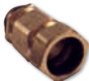
The E1FW gland range is designed for both multi-armour captive cone, providing an armour clamp and earth bond for steel wire, Braid and Tape armoured cable, to anchor and earth the armour of armoured cable to provide an inner flameproof / increased safety seal and an outer waterproof (to IP68) seal.
