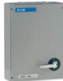
Exel 2 switch disconnectors and switch-disconnector fuses meet the constructional requirements for isolation of and are type tested to BS EN 60947-3. Switches are of the quick make and break type, suitable for use on AC or DC. Units have removable moving contact assemblies to facilitate wiring.
